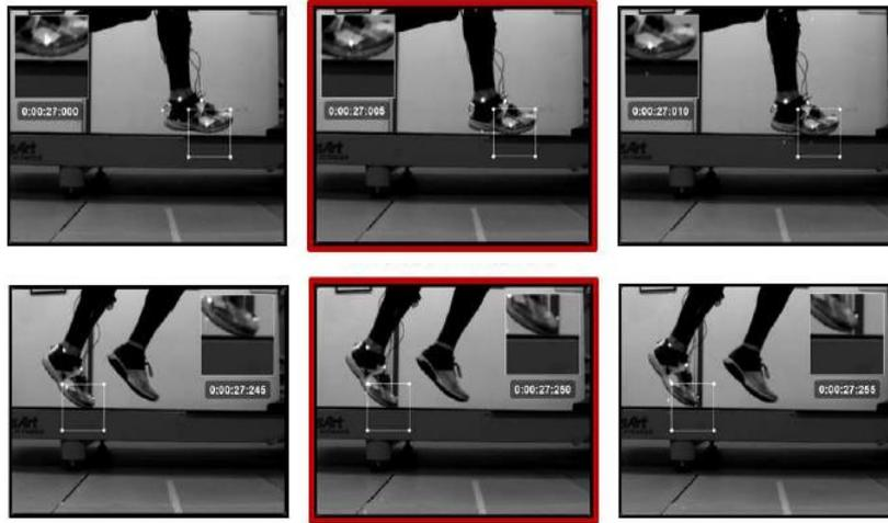
Figure 3: Determination of IC and TC timings using the 2D high-speed video camera. IC (upper pictures) is the first frame where the pixels representing one shoe are directly in contact with those representing the belt of the treadmill. TC (lower pictures) corresponds to the last frame where the pixels of the shoe are in contact with those of the treadmill.
