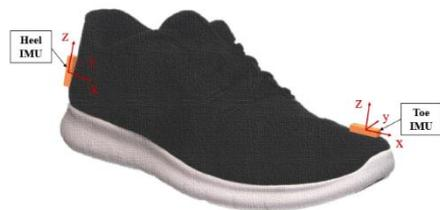
Figure 1: Schematic illustration of the position of the IMU sensors used in the proposed algorithm, including the three local axes (X-axis, Y-axis, and Z-axis). The two sensors are placed on the right shoe at the level of the first distal phalange (toe) and at the calcaneus (heel).
