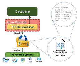
Fig. 3. Cemaden's Syntactic Integration Architecture
