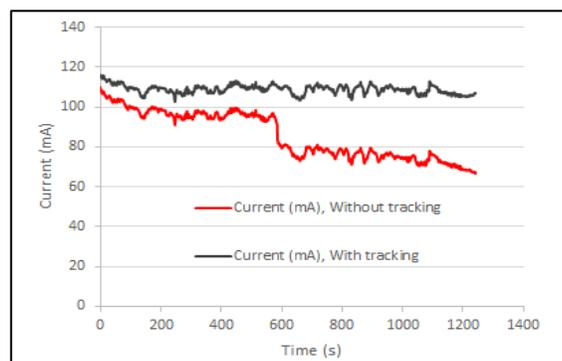
Figure 7: Current Performance of the Dual Axis Solar Panel Tracker in Comparison with the Single Axis Circuit
