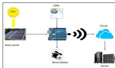
Figure 3: Tracking System Block Diagram
