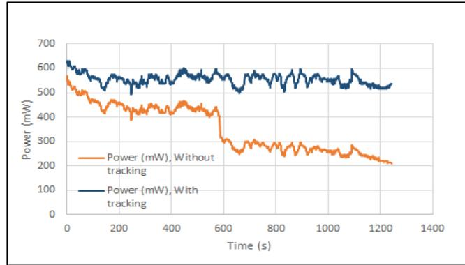
Figure 8: Power of the Solar Tracker Circuit Comparison with Single Axis Power Performance
