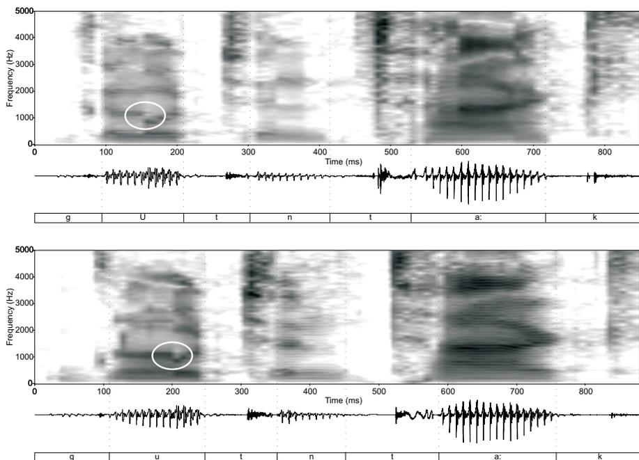
**Fig. 3.** A comparison of synthetic waveforms and spectrograms of a German sentence “Guten Tag.” when using fenemes (top) or triphones (bottom) as speech units. White oval shows an example of a within-phoneme formant discontinuity typical for feneme-based synthesis. Dotted lines show phoneme boundaries in the synthetic speech.
