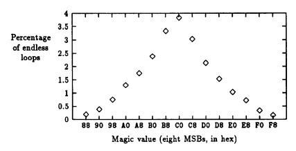
Fig. 2. Percentage of endless loops for the different 'good' magic values. Only the 8 MSBs of each magic value are indicated, the 24 LSBs are all zero.
