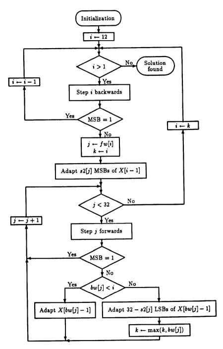
Fig. 1. Flowchart of the collision search algorithm
