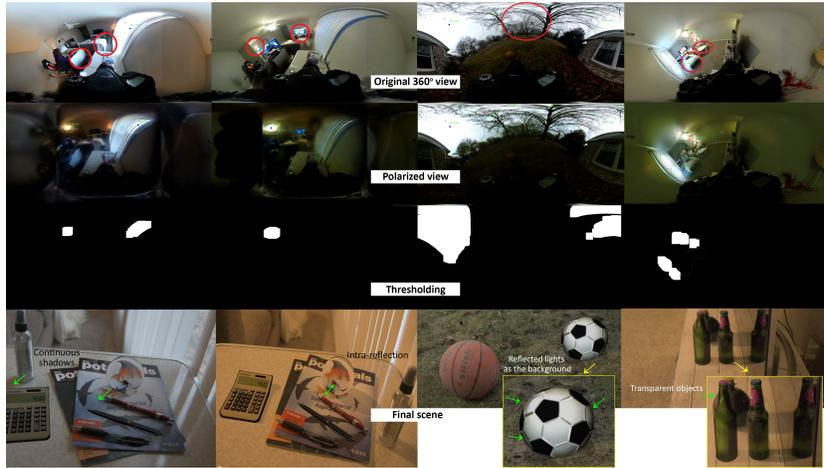
**Fig. 5.** System results with different lighting conditions and locations where each case has: (1) Original 360° view ”the red circles indicate the locations of unwanted reflections and glares mistaken with light sources”, (2) the view after polarization, (3) Threshold with minimal requirements, (4) the final image of the scene.
