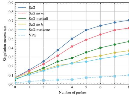
**Fig. 4.** Singulation success rate for different baselines.
