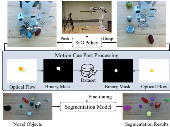
**Fig. 1.** The robot agent learns a Singulation-and-Grasping (SaG) policy via deep Q-learning in simulation. We collect the RGB images before and after applying the actions and use coherent motion to create pseudo ground truth masks for the segmentation transfer learning.
