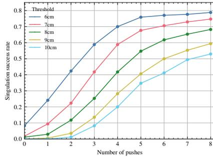
**Fig. 3.** Singulation policy performance with different distance thresholds.
