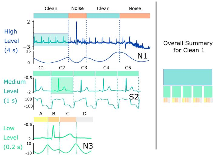
**Fig. 1.** Example of a multi time scale segmentation of a simple ECG signal with noise. The signal is from the Physionet[5]. Each row of signals indicates a smaller time-scale, zooming-in a specific sub-segment of the previous segmentation. On the right, an example of how we could summarize the first portion of the signal with this type of segmentation.
