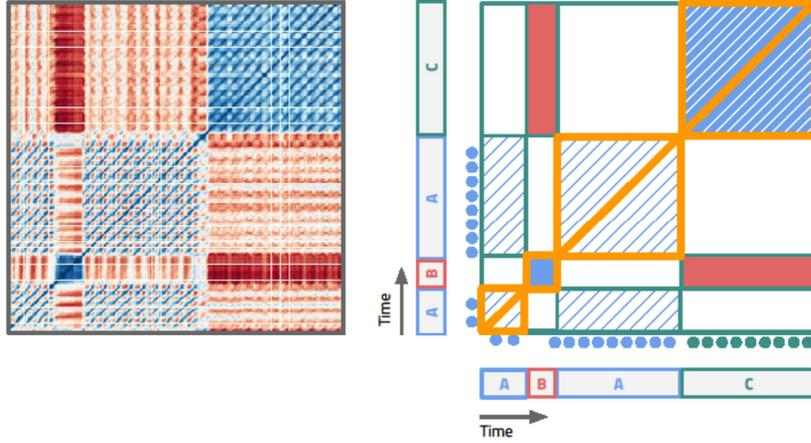
**Fig. 3.** At the left is the SSM designed from the signals acquired while an operator was performing 2 different workstations. At the right is a simplification of the original SSM, with highlights on the main structures present (Blocks and Diagonals).  $A$  being workstation 1 and  $C$  workstation 2.  $B$  is the interruption in the working line.[3]
