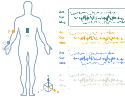
**Fig. 2.** Schematic of the placement of Inertial sensors, used for the dataset acquisition protocol. Based on [1] and [3]
