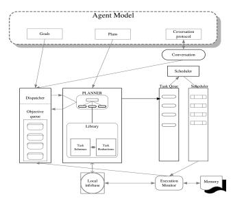
Figure 2, The Internal Architecutre of Intelligent Agent
