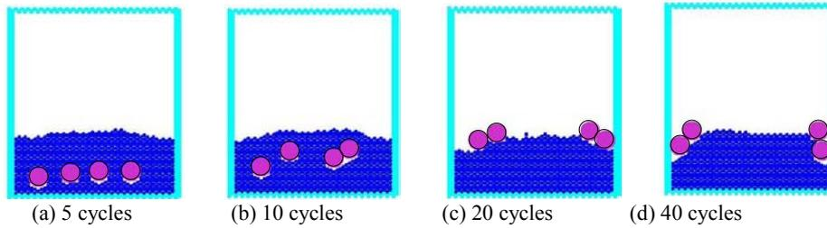
**Fig. 14.** Simulation result of small-medium particle segregation
