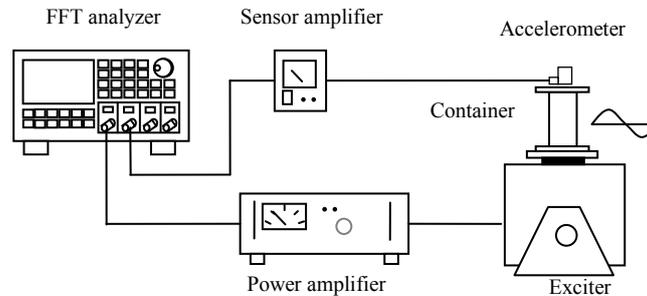
**Fig. 1.** Experimental setup of size-segregation of grains.
