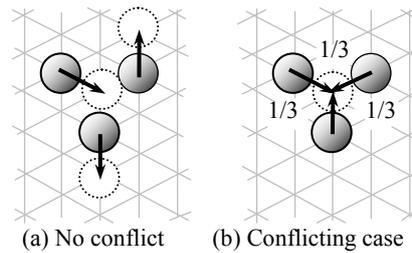
Fig. 6. Examples of rule for small particle movement
