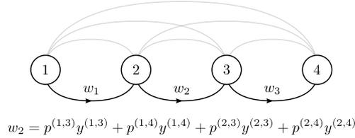
**Fig. 4** Number of passengers on the local service traveling between adjacent stops.
