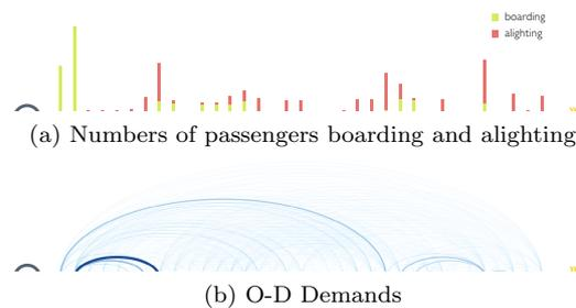
**Fig. 5** Visualization of the optimal limited-stop service route together with (a) numbers of passengers boarding and alighting at each stop and (b) O-D demands.
