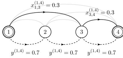
**Fig. 3** Example flows of passengers on O-D pair (1, 4) on both local service and limited-stop service serving stops 1,3, and 4.
